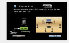
• If the measured level is within the 72 to 78 dB range, the level indicator is green.
